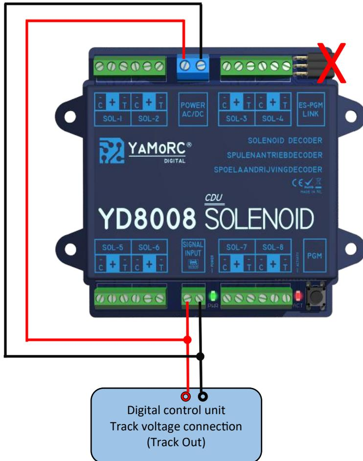
Power supply of the YD8008 via a separate power supply unit (DC) or a transformer (AC) with min. 500 mA output current
